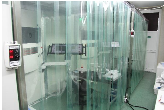
20 and 30 cm diameter IBS coating chambers
